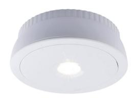
The Elled Emergency Downlight surface or recessed mounting enclosure houses an 'intelligent' ProSeries DALI/Self-Test LED driver and a Lithium Iron Phosphate (Life) battery. A Nichia '3 watt' high power white LED is mounted in the fascia plate in conjunction with a choice of wide angle or 'corridor' distribution lens.
